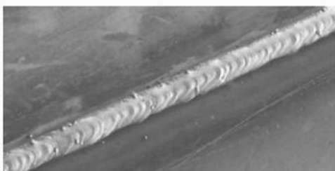
4mm carbon steel plate angle welding performing
