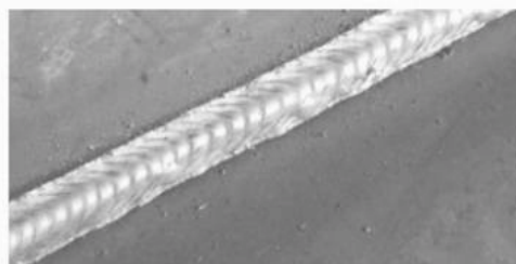
220V 6mm steel plate angle welding
